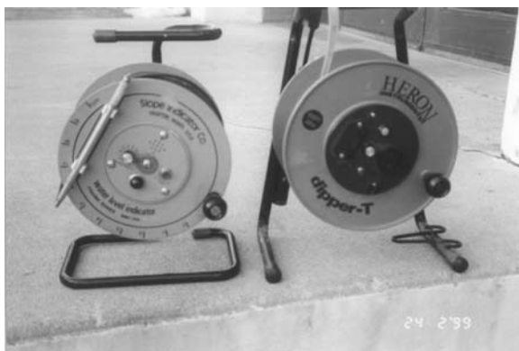
Figure 26.13 Batteries located on the reel housing provide good design.
