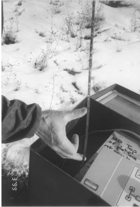
Figure 26.5 Level measurement taken with a steel tape. The “wet” mark is accentuated by a carpenter’s chalk.
