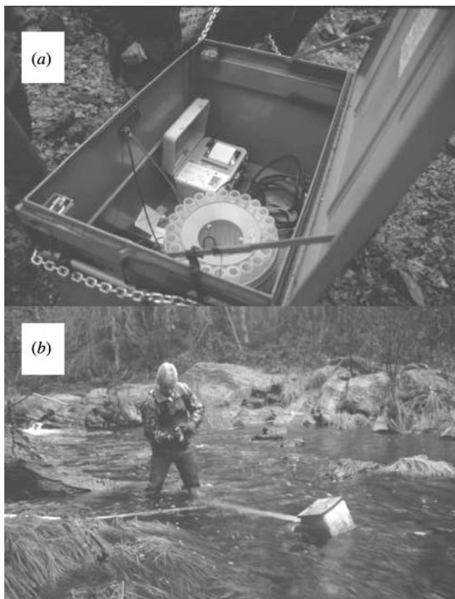
Figure 25.4 (a) Automatic pump sampler deployed in a locked, steel box chained to a tree to prevent theft and loss during high-flow events. A flowmeter was utilized to activate pump the sampling sequence during storm events. (b) Sample tube inlet attached to a floating boom anchored to the stream bottom. Tube inlet was located at a position along the boom to maintain inlet at 0.6 depth. Sampling tube was enclosed in a rigid PVC tube anchored to bottom to prevent debris from collecting and disturbing sampling tube.
