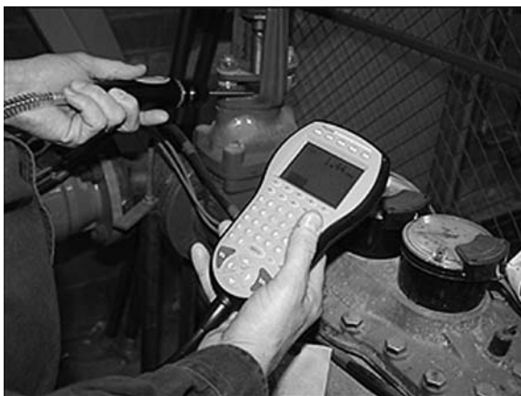
Figure 16.2 Hand-held analyzer (sniffer).
