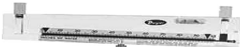
Figure 11.1 Old-style portable instrument (inclined manometer).
